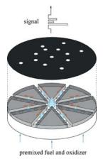
Figure 1. A cartoon of an Infofuse in which patterns of emissive salts transmit information as pulses of light of different wavelengths.
